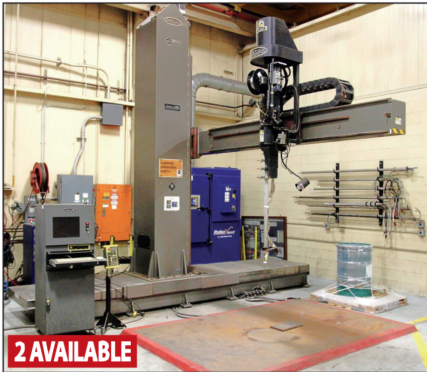
AMET CBMF 3 X 2.5 ADVENT-BR-FX BORE CLADDING WELDING SYSTEM
