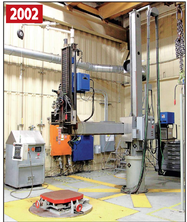
ARONSON 2G10VRA10CL-PK WELDING MANIPULATOR SYSTEM
