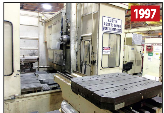
GIDDINGS & LEWIS 450 SERIES MC50 CNC HBM
