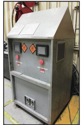
PDS-BARTECH 30.1343 INDUCTION HEATER SYSTEM
